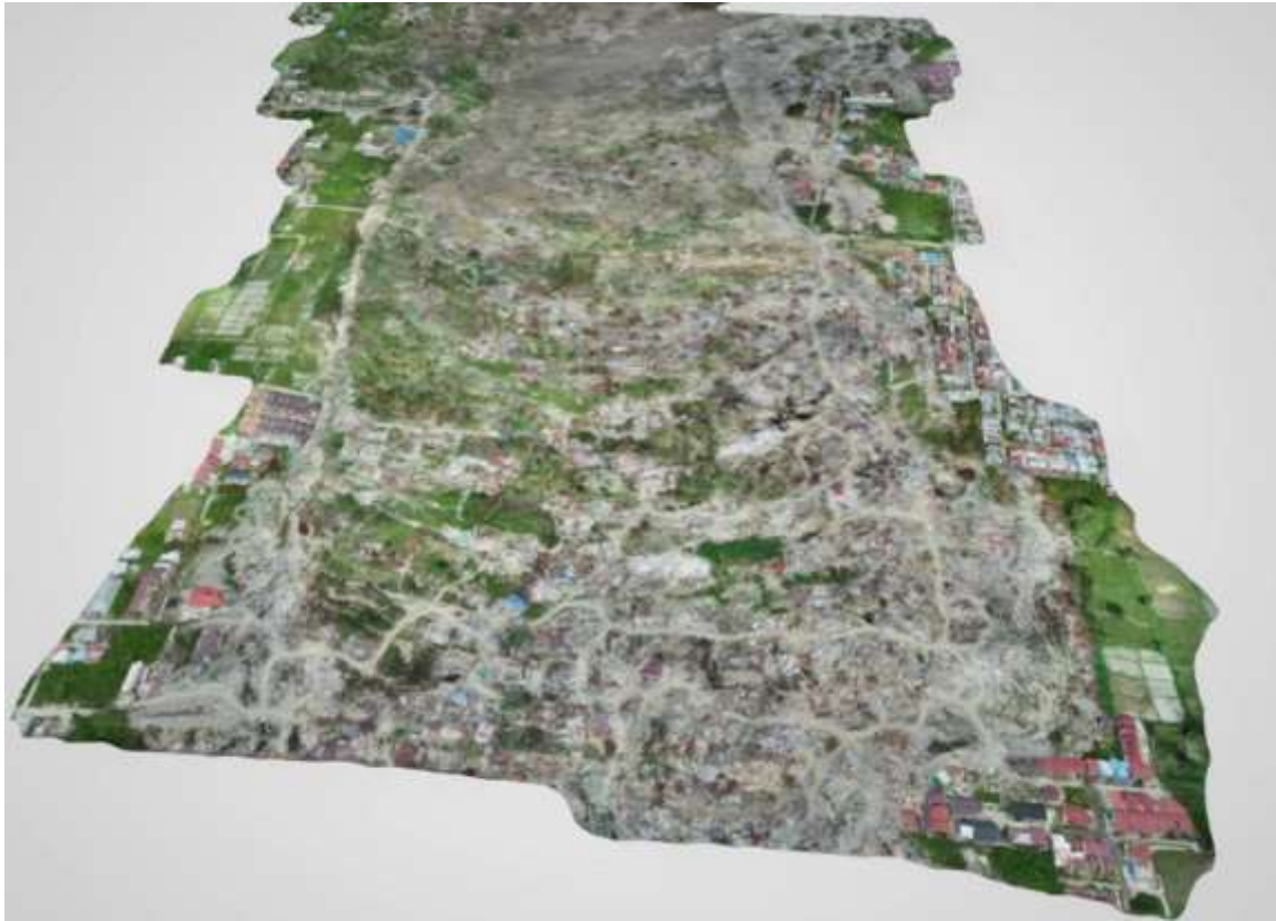
Figure 40: Partial 3-D Image of Petobo Sub-district lateral spreading developed from 3750 drone images using “Structure-from-Motion”.
