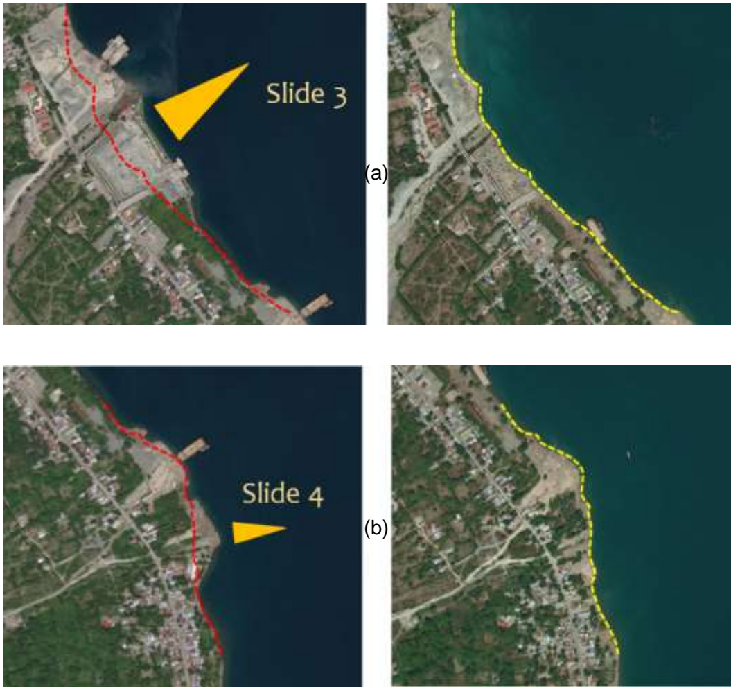
Figure 12: DigitalGlobe images of the location of (a) Slide 3 (0.801S, 119.806E) and (b) Slide 4 (0.808S, 119.811E), before (left) and after (right) the earthquake.
