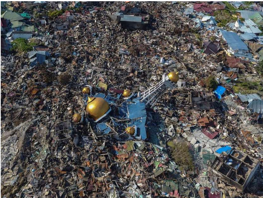
Figure 38: Aerial image of accumulated building debris, including a mosque, at the base of the Balaroa neighborhood slide (Photo Credit: Antara Foto/ Hafidz Mubarak A/Reuters).
