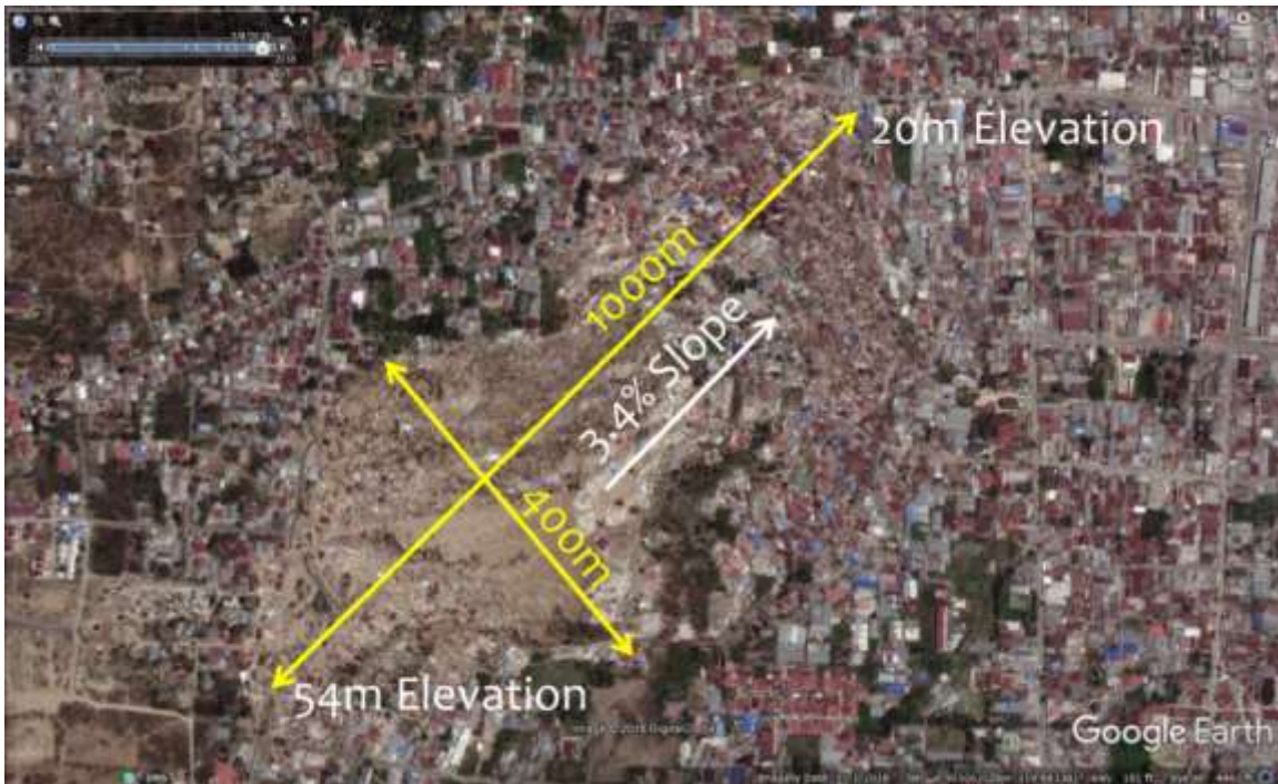
Figure 36: Google Earth image of Balaroa Neighborhood before earthquake (top) and after earthquake (bottom) showing extent of lateral spreading due to liquefaction.
