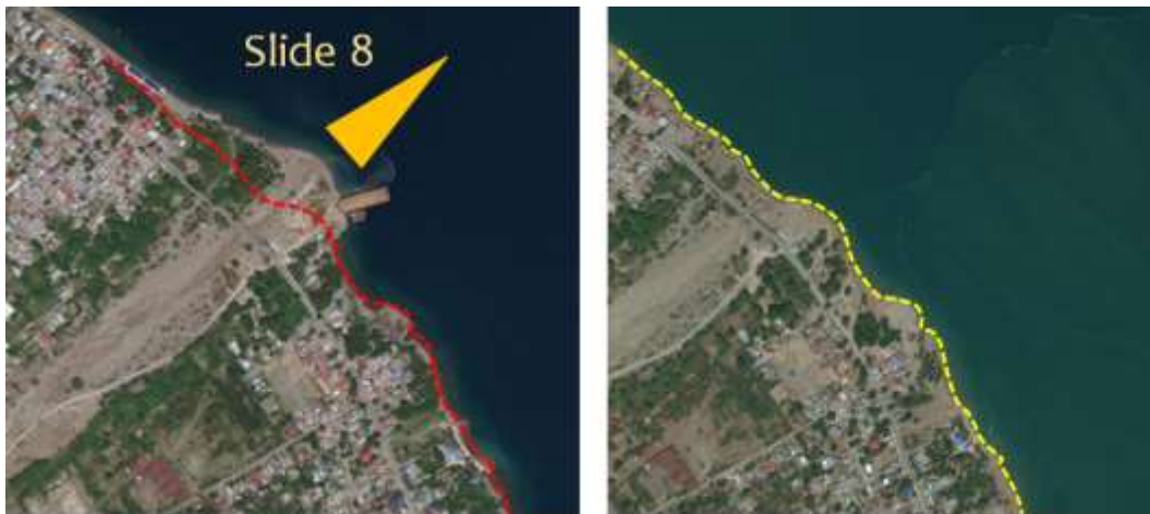
Figure 15: DigitalGlobe images location of submarine landslide 8 ( 0.846\text{S}, 119.823\text{E} ) before (left) and after (right) the earthquake.
