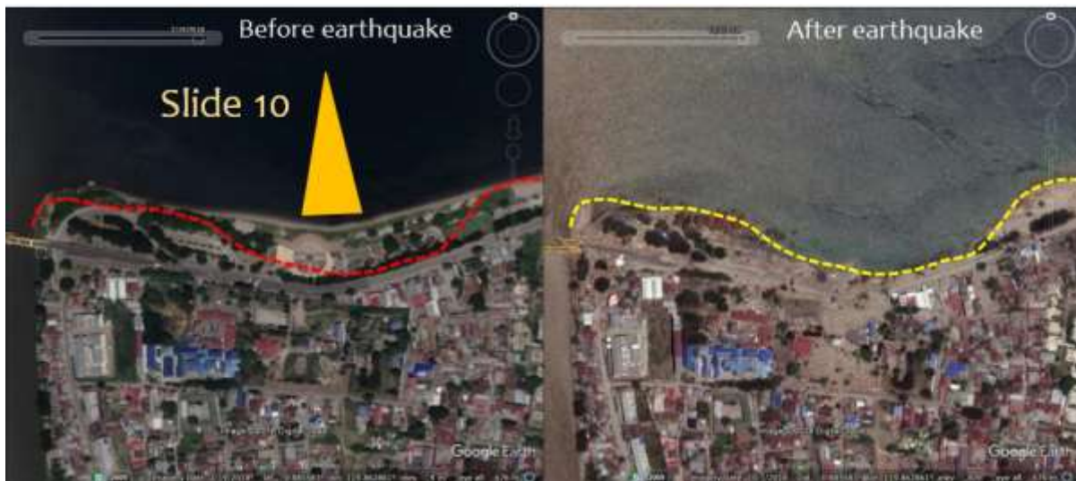
Figure 20: Google Earth images of the location of Slide 10 on the South shore of Palu Bay East of the Palu River mouth (0.8855S, 119.863E) before (left) and after (right) the earthquake.
