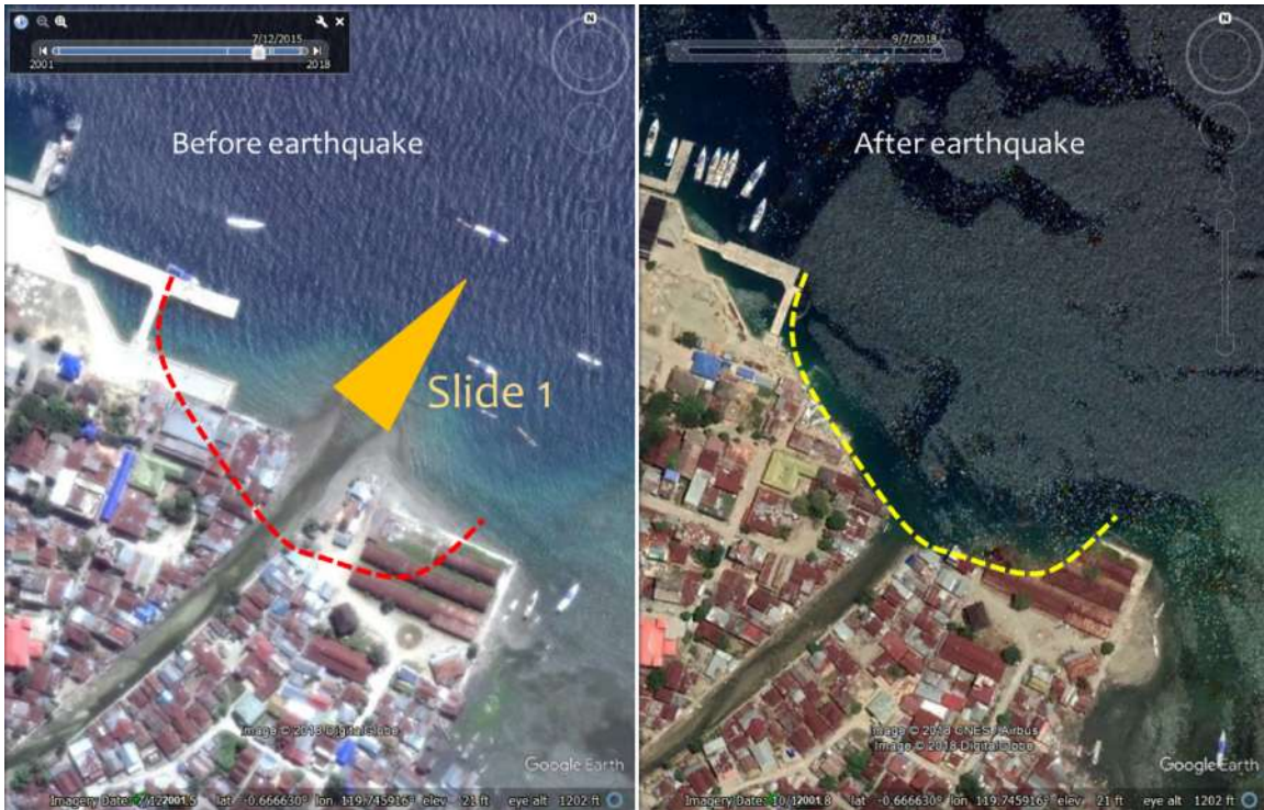
Figure 9: Google Earth images of the location of Slide 1 in Donggala town (0.667S, 119.746E) before (left) and after (right) the earthquake.
