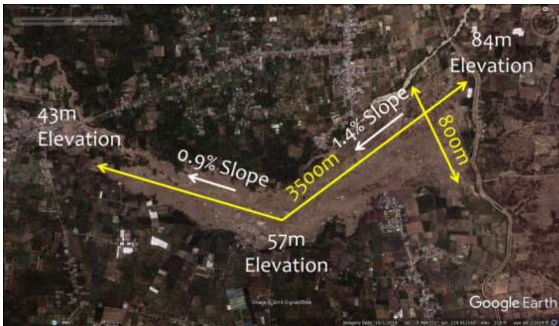
Figure 42: Google Earth image of Jono Oge Village before earthquake (top) and after earthquake showing extent of lateral spreading due to liquefaction (bottom).
