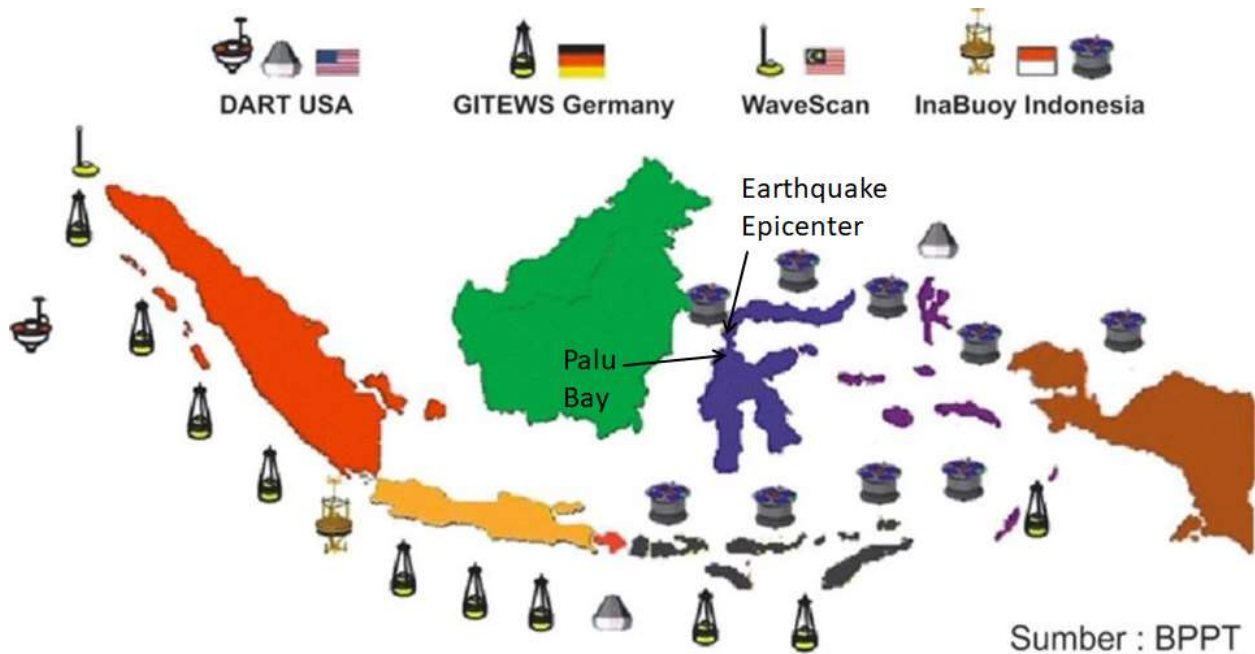
Figure 27: Graphic showing location of tsunami buoys around the Indonesian Islands (Source: BPPT, Indonesian Agency for the Assessment and Application of Technology).
