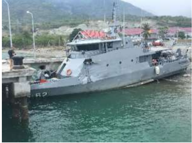
Figure 70: Naval ships in Watusampu Naval Base beached (left) and damaged from pounding against piers (right) because of tsunami waves.
