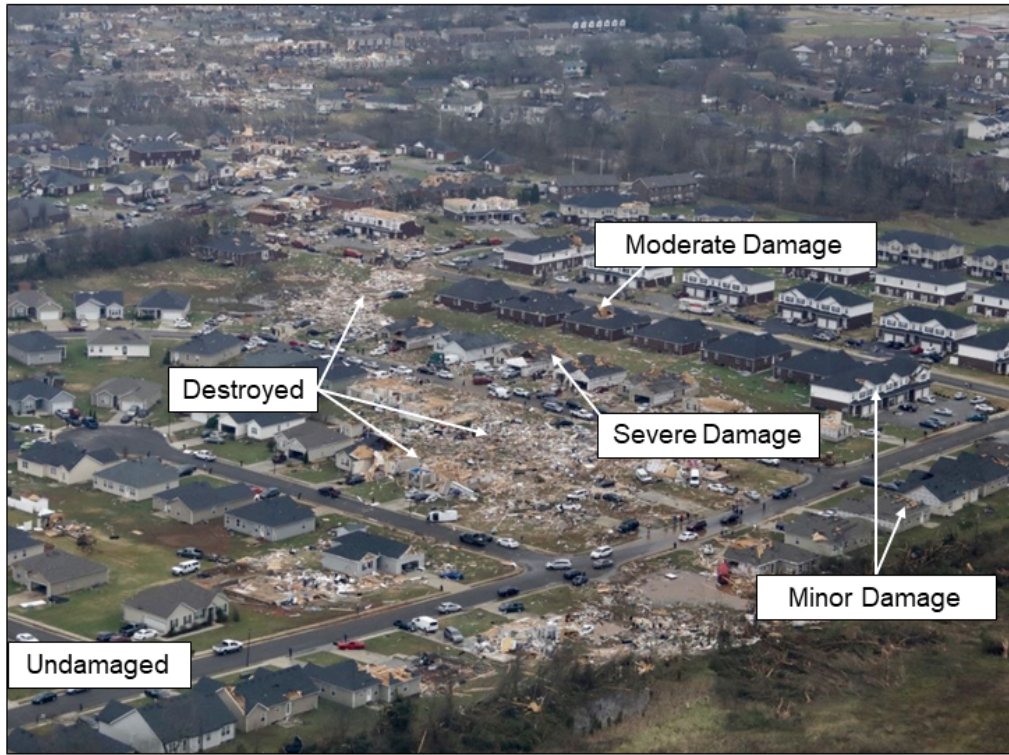
Figure 6.1.1. EF-3 tornado track through Bowling Green highlighting damage gradient to either side of the track (source: CNN news Clinton Lewis )
