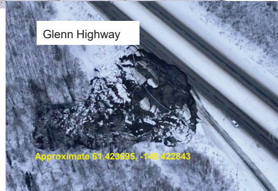
Massive coseismic landslide (length= 100 m, width =70 m) in Glenn Highway, AK following the Alaska earthquake (photo modified from AP)
