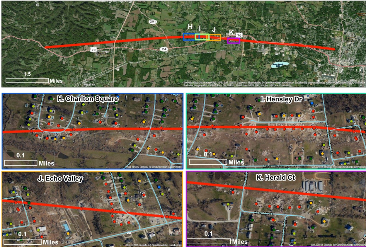
Figure 5.2. StEER FAST D2D assessments in response to the Nashville tornado in key geographic regions relative to the tornado centerline. Blue lines in the detail plots indicate routes captured with streetview imagery.
