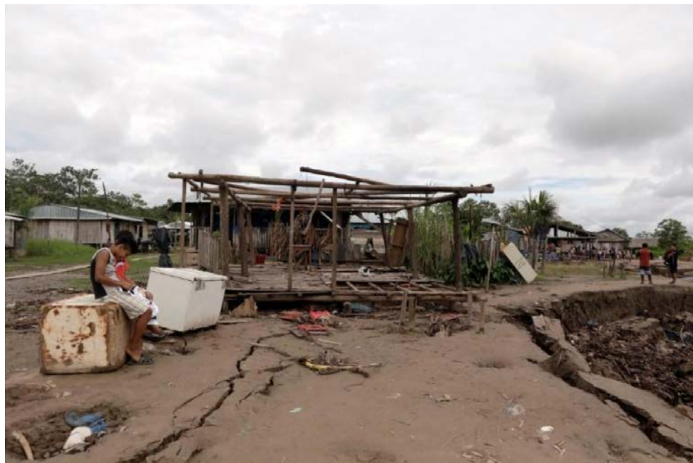
Figure 9.11. Lateral spreading along the Huallaga river at the Santa Gema near Yurimaguas in the Amazon region of Peru, (Jourdan et al. 2019).
