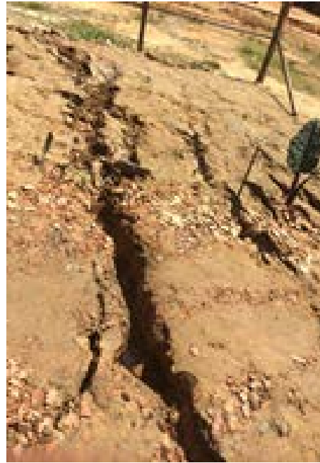
Figure 9.32. Seismically-induced ground damage at El Sauce District (Source: Ministerio de Vivienda del Perú - Photo by Miguel Estrada).
