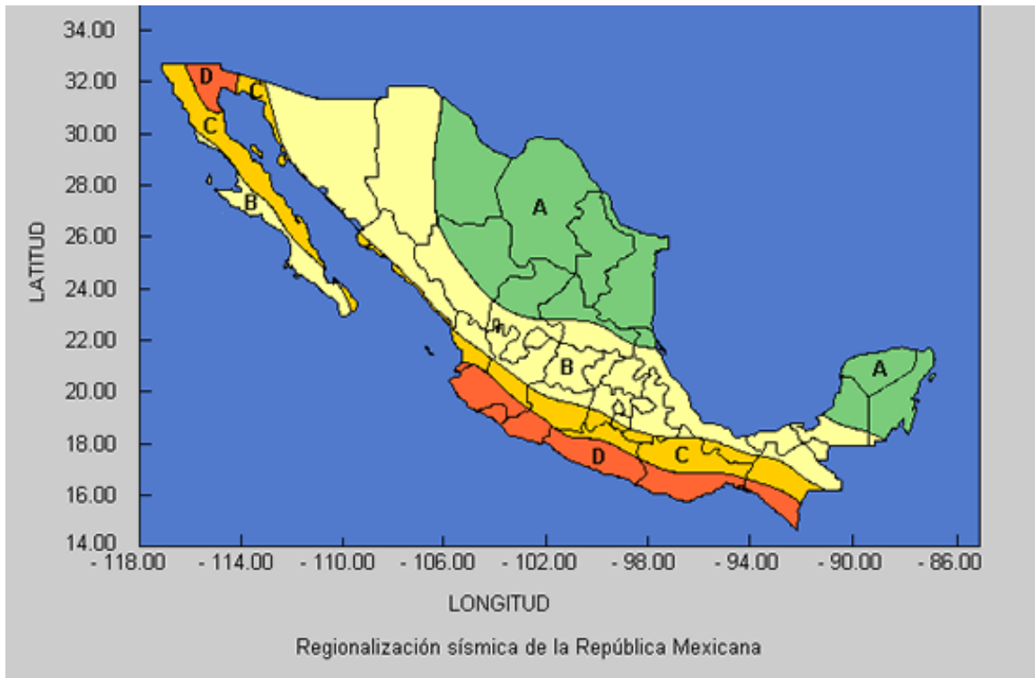
Figure 5.1. Seismic zonation of Mexico according to the 1993 edition of the Manual for Civil Works of the Federal Commission Electricity (MOC-CFE, 1993).
