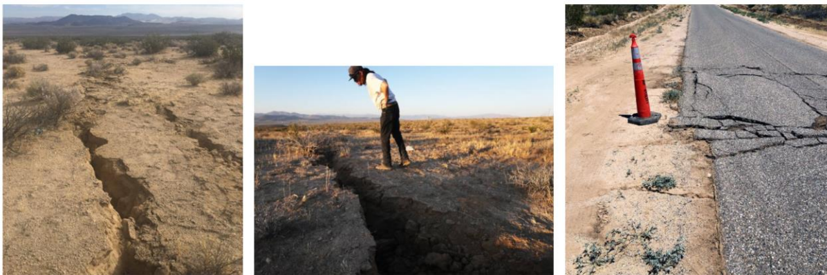
Figure 44. Surface Fault Rupture following M 6.4 Ridgecrest earthquake (a) Off the road rupture (reported by Emily Guerin 43 ), (b) Ground crack near Ridgecrest 44 , (c) fault rupture across Randsburg Wash Road to the south of State Route 178, measured offset of approximately 1.5 feet (457 mm) (Source: Brian Olson Twitter page 45 ). All images reported in the VERT report, Appendix B.
