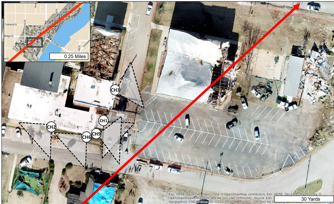
Figure 7. Locations and viewing angles of security camera footage obtained by the FAT overlaid on the post-tornado aerial imagery. Red arrow indicates the approximate centerline of the tornado path based on the damage in this area.
