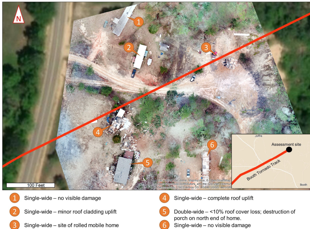
Figure 21. Orthomosaic of the tornado path through a mobile home community just north of Booth, AL. The tornado path appears to have been only a few yards wide at this point.
