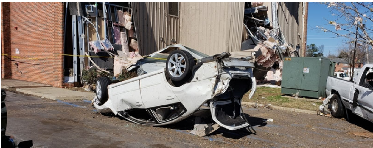
Figure 18. Nissan Sentra (Vehicle 4 in Figure 17) flipped by the tornado. Final resting location was approximately 80 ft from origination point in the direction the tornado traveled.
