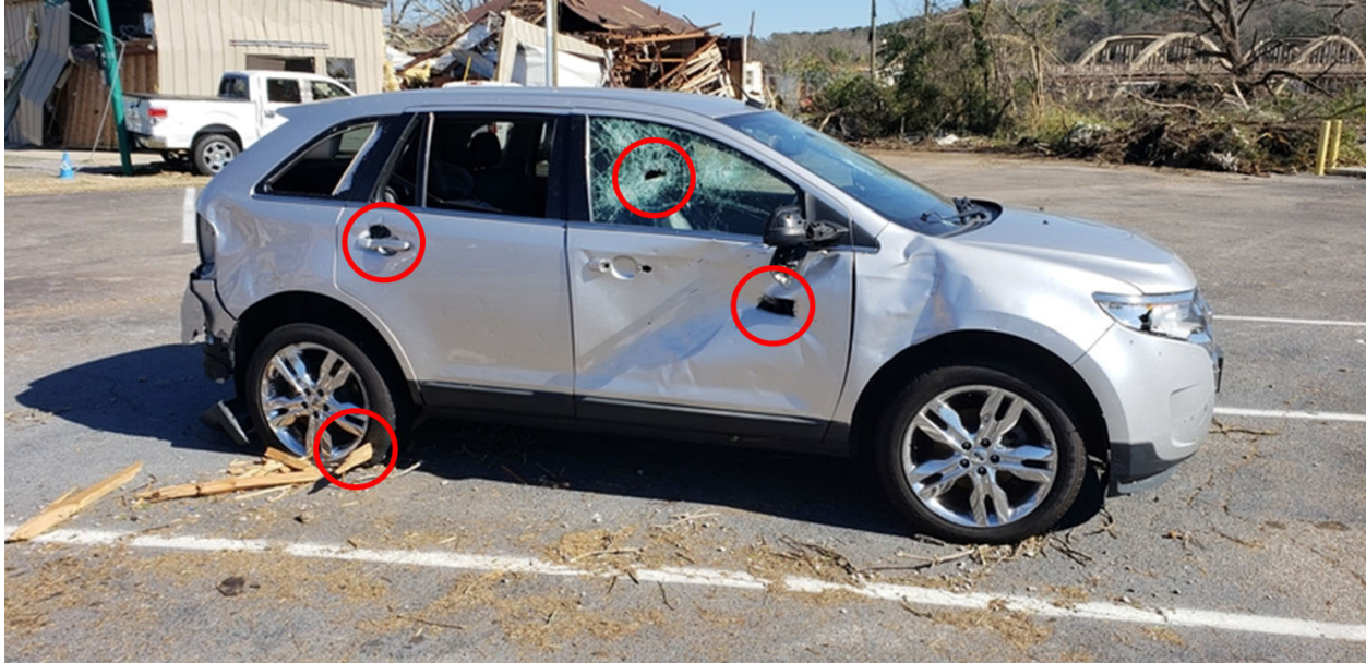
Figure 19. Wind-borne debris pierced doors and windows of this midsize SUV in multiple places.
